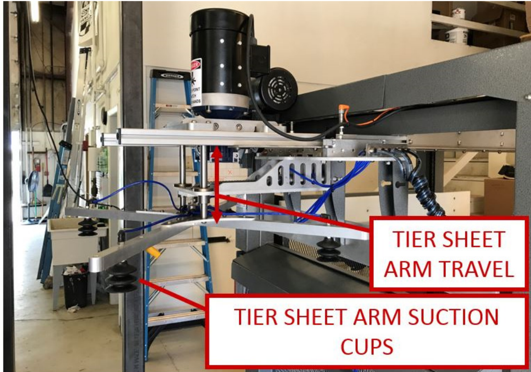
Figure 13 Tier Sheet Arm Mechanism
